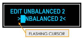
5. Each character may be changed by scrolling through the available character list using the ▲UP and ▼DOWN Buttons. When the desired character is reached, move the cursor using the ◀LEFT or ▶RIGHT Buttons to change another.
